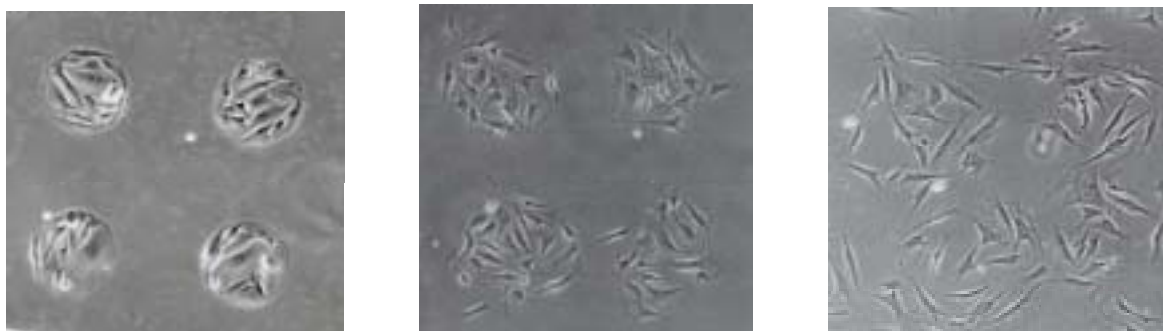
Fig. 5.2. Example of a dynamic substrate that can be electrically switched to turn on cell migration. Cells were initially patterned on circular regions and maintained in culture ( left ). Application of an electrical potential to the substrate switched the surrounding regions to a state that promoted cell migration.
