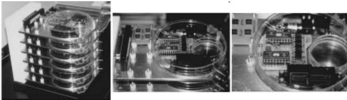
Fig. 6.5. Novel device for applying specific regimens of mechanical and/or electrical stimulation to engineered tissues in vitro developed in the laboratory of R. Dennis (University of Michigan). Left. The system is modular and is designed to operate in stacks of 6 units per tower in an incubator. Center. The system uses standard cell-culture disposable plastic dishes. Individual tissue constructs are grown in 35 mm-diameter culture dishes. A 100 mm-diameter culture dish houses the tissue in the 35 mm culture dish, a servo motor, a force transducer, a stepper driver, a high-voltage bipolar stimulator, and two microcontrollers. The units are interchangeable and connect with the main power and data bus via a 25-pin D-sub connector. Right. A close up view of the prototype device, showing the force transducer in the foreground in the 100 mm dish, the servomotor in the background, and the electronics module to the left of the 35 mm culture dish. The mounting fixtures for the tissue construct and the electrodes are not shown. Micropower techniques have been employed to minimize power dissipation and heat accumulation (R. Dennis; used by permission).
