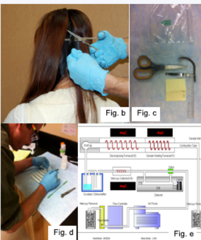
Fig. b: Demonstration of hair collection site and general method. The hair is usually wrapped in a sticky note, paperclipped, then stored in a plastic bag (Fig. c). Fig. d: Preparing samples to be run through the analyzer. Fig. e: Diagram of the Nippon MA-2 direct mercury analyzer.
