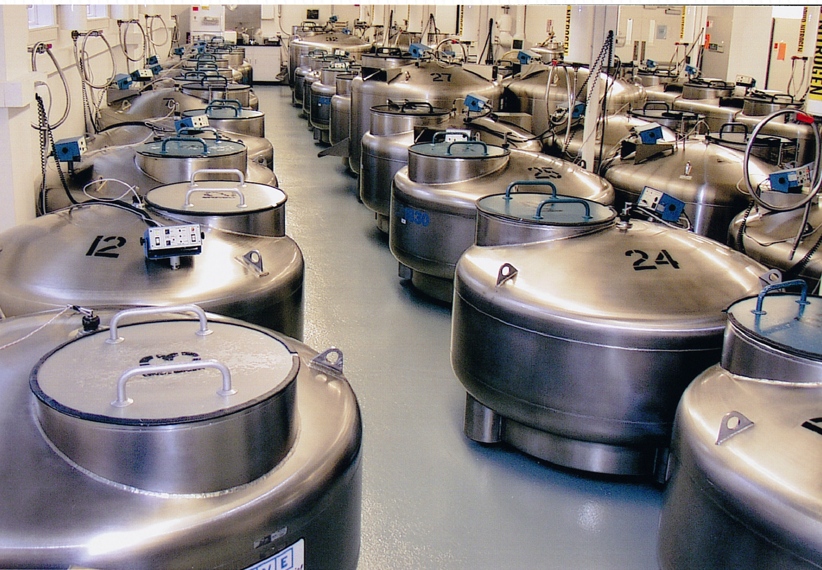
Figure 2-5. Established in 1953, the Coriell Institute for Medical Research distributes cell lines and DNA samples to researchers around the world. Shown here are Coriell's cryogenic tanks filled with liquid nitrogen and millions of vials of frozen cells. Credit: Courtney Sill, Ph.D., Coriell Institute for Medical Research.
